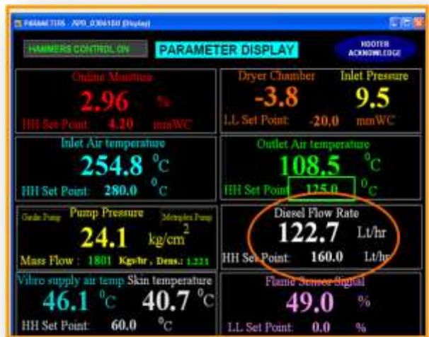
ONLINE DIESEL MONITORING
